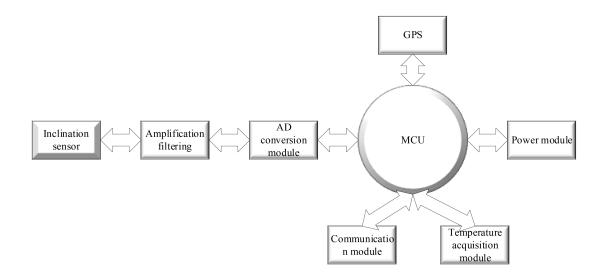
Figure 1. Overall hardware design of arc remote monitoring terminal.
