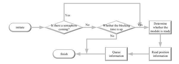
Figure 7. Software design flow of GPS module.
