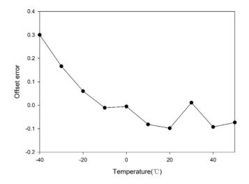
Figure 10. Temperature compensation between  $-40^{\circ}$ C and  $50^{\circ}$ C.
