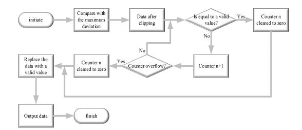
Figure 5. Digital filter design flow.
