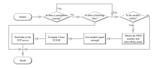
Figure 6. BC28 communication program design flow.
