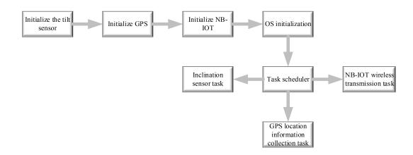
Figure 3. Overall design of remote monitoring terminal software.
