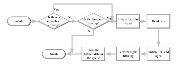
Figure 4. Data acquisition and processing task design of inclination sensor.
