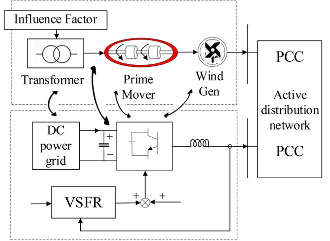
Figure 4. Schematic diagram of stability control structure.
