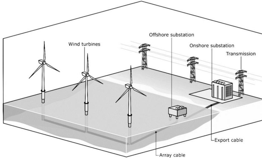
Figure 2. Topological model of offshore wind power system.
