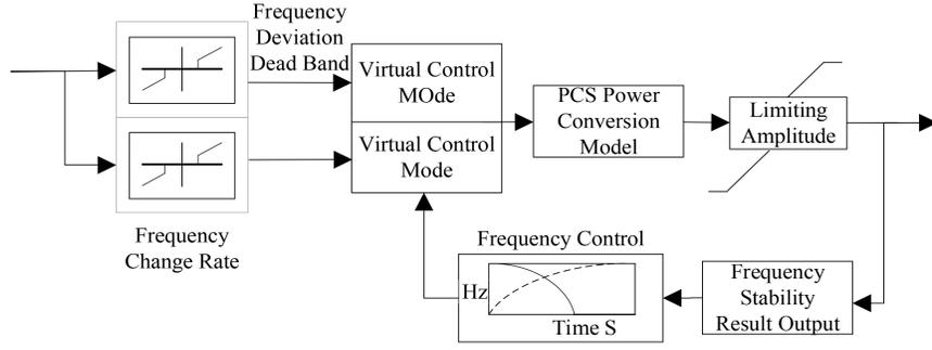
Figure 3. Schematic diagram of load frequency response model.
