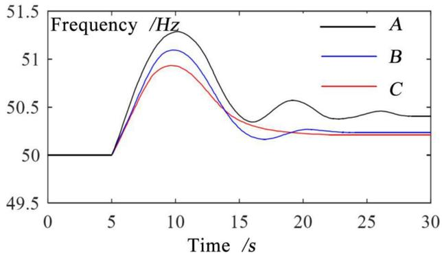
Figure 6. Frequency stability simulation results of different strategies.
