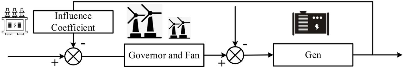
Figure 1. Frequency response transfer function model.
