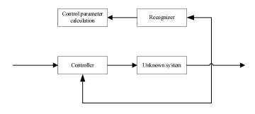
Figure 1. Automatic adjuster.
