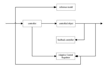
Figure 2. Model reference adaptive control.
