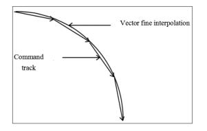
Figure 4. High-precision vector interpolation.
