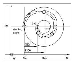
Figure 6. Vortex/conic insertion.
