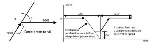
Figure 2. Optimal angular deceleration high-precision control mode.
