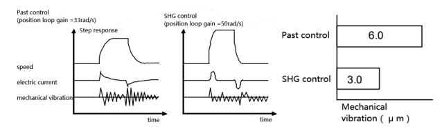
Figure 9. SHG control and mechanical vibration amount comparison.
