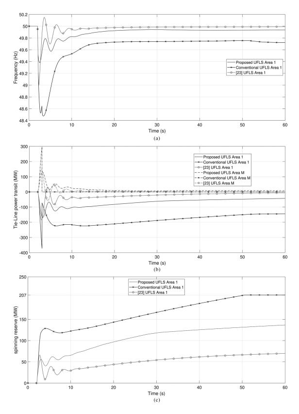
Figure 6. Frequency, tie-lines power transit, and spinning reserve in scenario 2: (a) frequency; (b) tie-lines power transit; (c) generated power in area 1.
