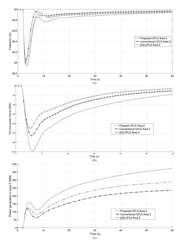
Figure 5. Frequency, tie-lines power transit, and spinning reserve in scenario 1: (a) frequency; (b) tie-lines power transit; (c) generated power in area 2.
