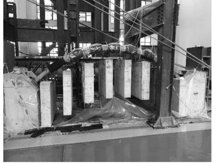
Figure 3. Accelerated corrosion scheme under weight load: (a) the weight design of the dead load and (b) accelerated corrosion test site.
