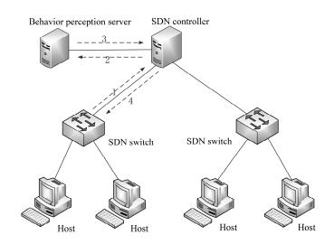
Figure 1. Network topology structure of SDN user behaviour perception system.
