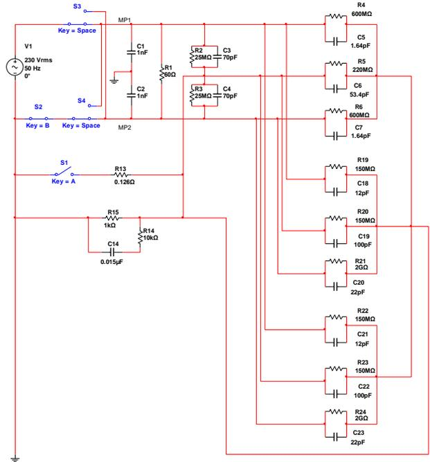
Figure 1. Electrical circuit model of a patient monitor for the simulation of equipment leakage current
