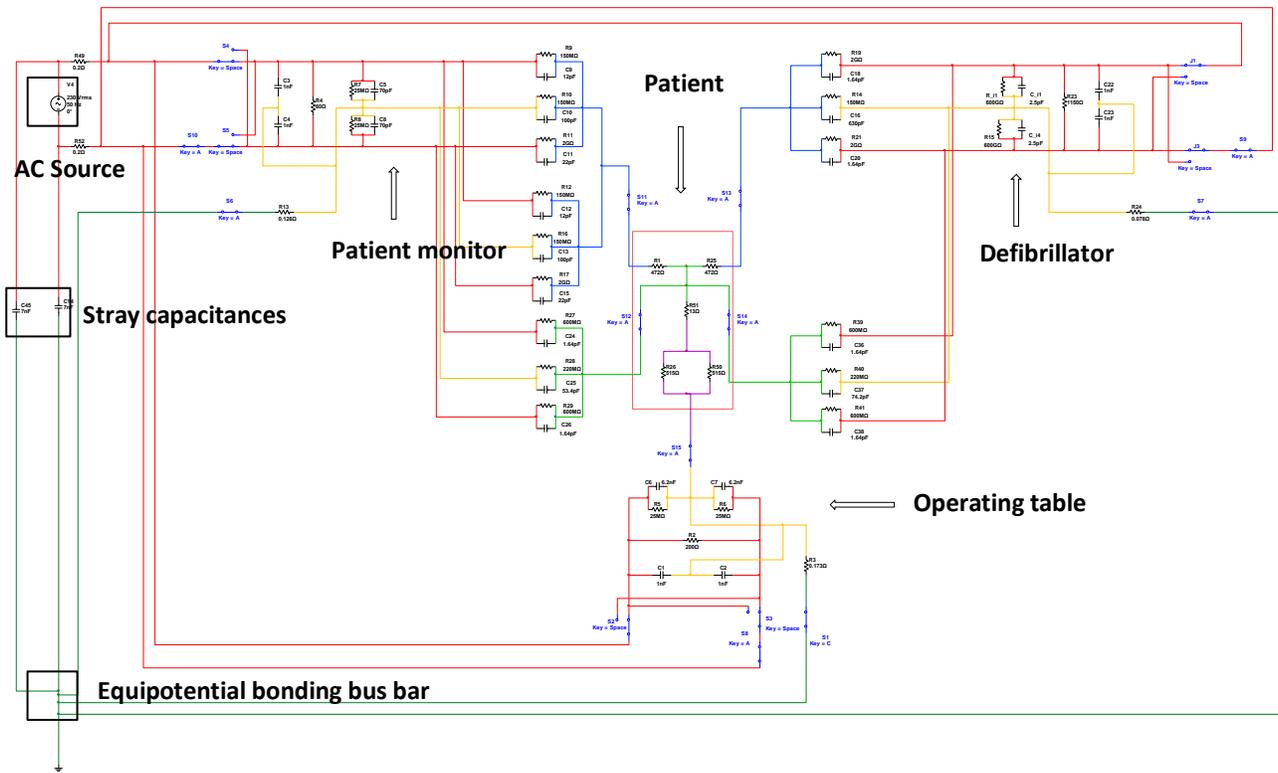
Figure 2. Electrical circuit model of three MEE in contact with the patient in an operating theatre
