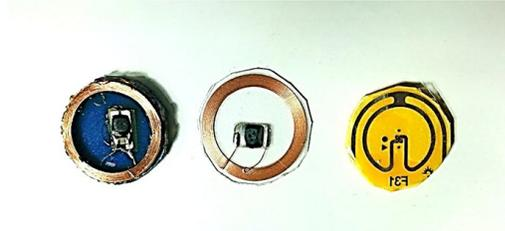
Fig. 1: Passive tags used in experiments. From left to right: LF, HF, and UHF
