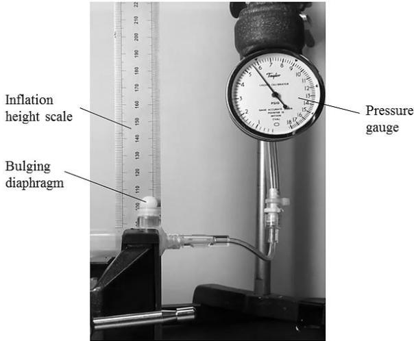
Figure 5 Experimental apparatus to evaluate the biaxial characteristics of latex rubber diaphragm at room temperature (21°C).
