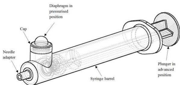
Figure 2 ProDural concept design with visual pressure drop indicator integrated into the distal end of the syringe barrel
