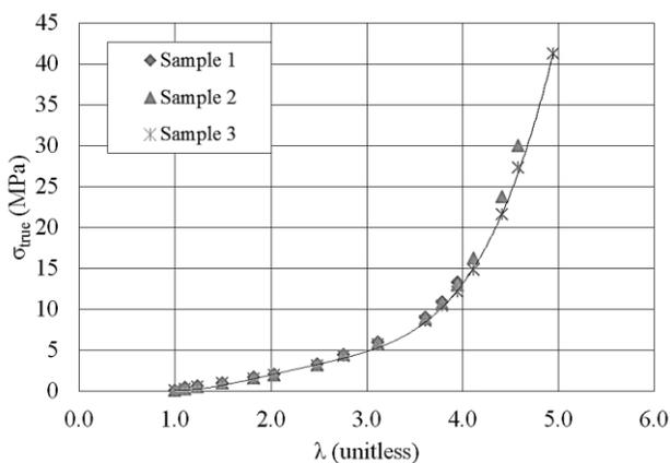
Figure 8 A graphic representation of the relationship between true stress and the stretch ratio.
