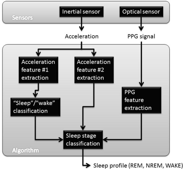
Figure 2 - Block scheme of the algorithm for automatic sleep profile estimation.
